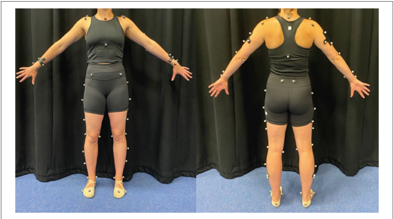
Figure 1. Placement of full body marker set used in this study.
