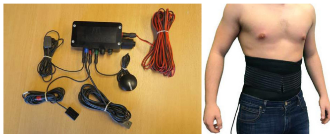
Figure 2 On the left is a photograph of the MAREC device and related connections and on the right the kidney belt containing a three-axis accelerometer worn by the participating operators.
