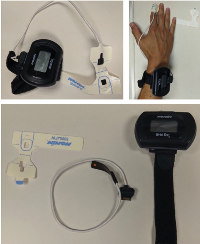
FIGURE 2 Pulse oximeters. The WristOx 3150 model (Nonin Medical) pulse oximeter is pictured alongside the adult flexible finger sensor (8000J) and accompanying disposable adhesive fastener. Photograph credit(s) Drs Johnson and Wheatley-Guy, and Mr Jesse Schwarz of the Johnson Lab, Mayo Clinic, Scottsdale campus in Scottsdale, AZ, USA.
