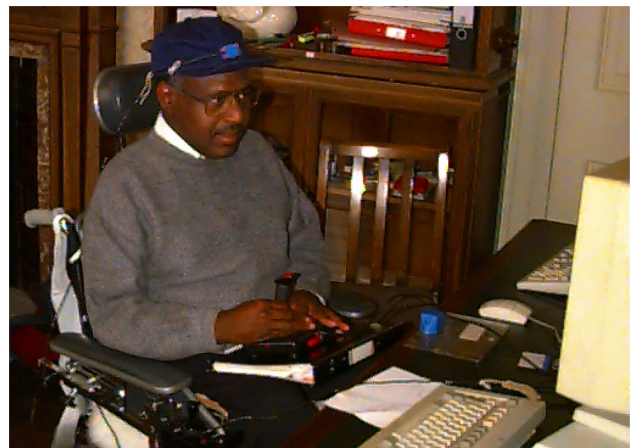
Fig. 1 Jester in use. Note the plastic cube mounted on the baseball cap for head gestures and the analogue joystick for hand gesture. Both could be used independently or combined
