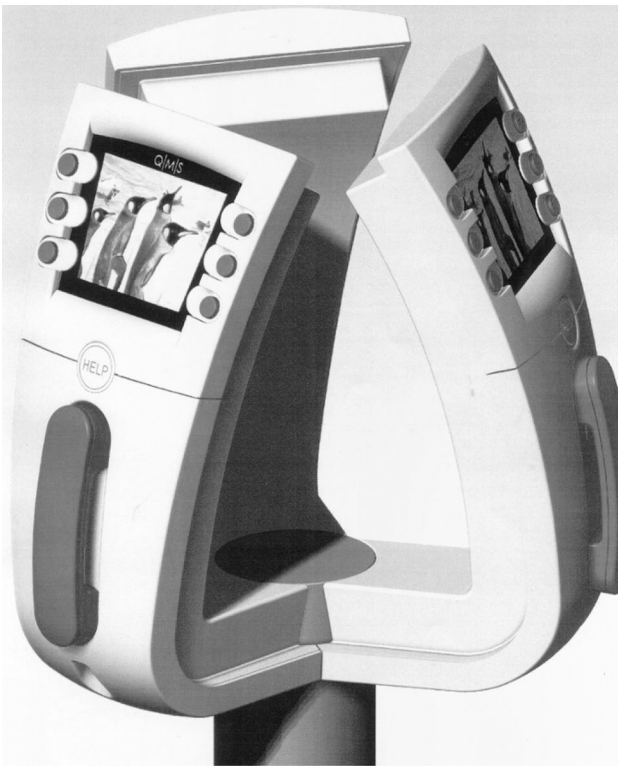
Fig. 5 Personal Information Point. Note the telephone handset for audio output, the LCD screen for visual output, and the six buttons arranged either side of the screen for input. To use the PIP, the user would have to be able to see the screen, hear the audio, and simultaneously hold the handset and press the buttons
