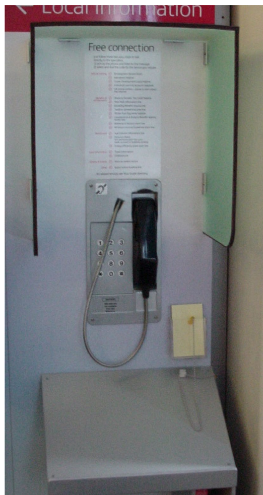
Fig. 7 The Your Guide telephone. Note the cable obscuring the sunken, rubberized buttons, and the black foam rubber bumper around the plastic shroud to protect against people bumping their heads on the hard plastic
