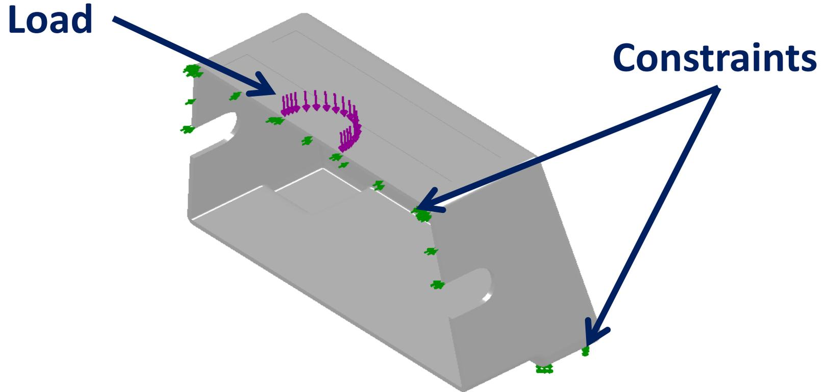
Model split symmetrically. Force of 300 N with a 50mm radius semicircle or displacement of 13mm applied. Constraints to feet stabilised using springs.
