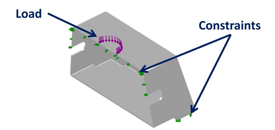
Model split symmetrically. Force of 300 N with a 50mm radius semicircle or displacement of 13mm applied. Constraints to feet stabilised using springs. <sup>12</sup>
