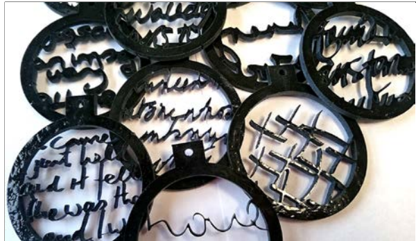
Figure 19. AWJ-cut medal on black soda lime glass
