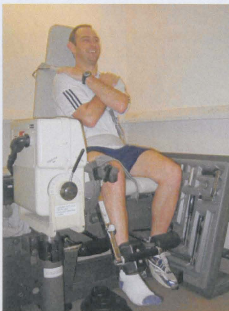
Figure 4.2 – Position of participant in the Cybex II isokinetic dynamometer during isokinetic assessment of the knee extensors and flexors
